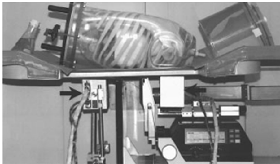
Fig. 19 PEM detectors installed on an autopsy system [42]
